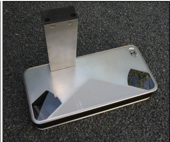
Figure 5. A camera hidden under the mast views two optical paths to tilted mirrors under the glass at each corner. The path to the lower left corner is enabled by the mirror at the center back that redirects half of the camera view. Together, the mirrors allow the single camera to simultaneously achieve two views of the wire.
