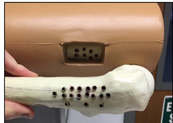
Figure 7. The surrogate bone is shown here, with 17 small diameter brass tubes inserted to provide reproducible wire placement.
